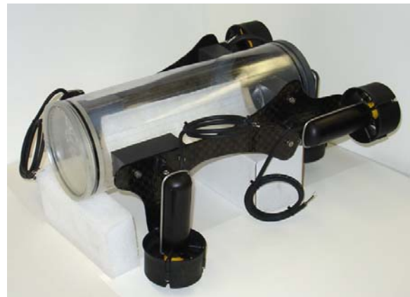
Figure 2: Platform body and thrusters
