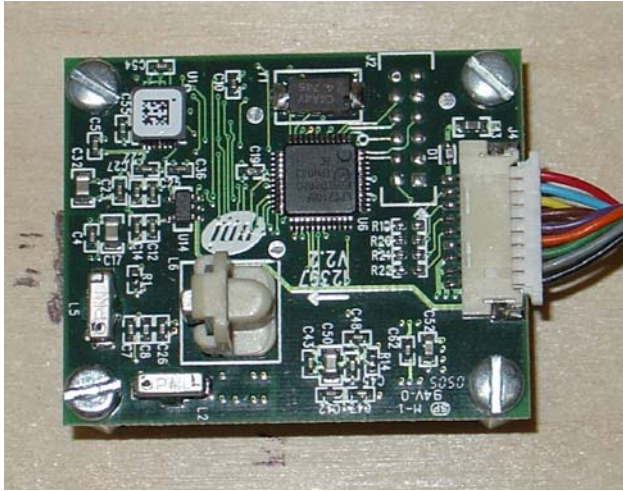
Figure 5: Precision Navigation TCM5 Compass throughout its operational range. This sensor interfaces with a serial port on an Atmel microcontroller.
