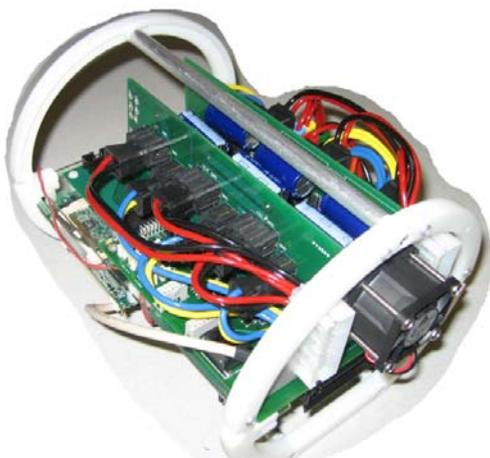
**Figure 2 - Drive Electronics with Backplane**
