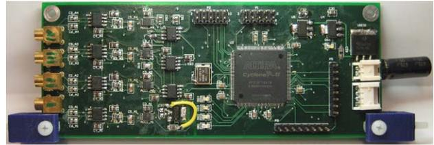
**Figure 7 - Hydrophone Signal Processor**
