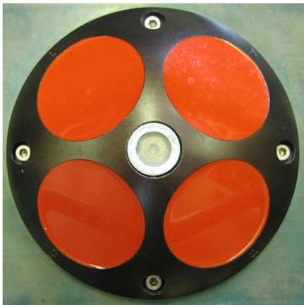
**Figure 4 - Doppler Velocity Log Transducer**
