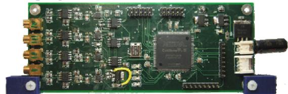
**Figure 11 – Hydrophone Signal Processor**
