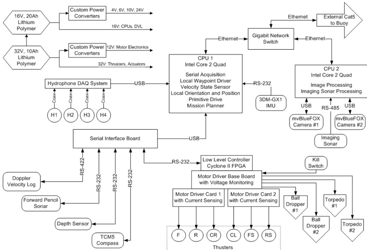
**Figure 2. SubjuGator System Diagram**
