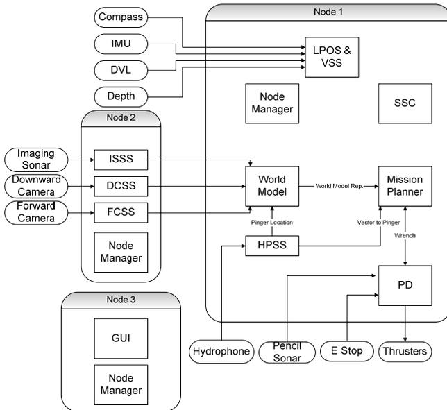
**Figure 12. Software Architecture**
