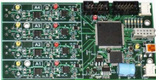
**Figure 11. Hydrophone Signal Processor**
