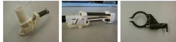
Figure 13: Left: Ball dropper, Middle: Torpedo shooter, Right: Manipulator.
