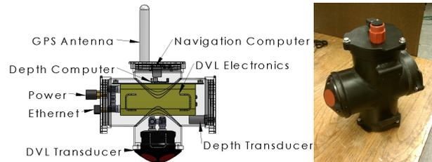
Figure 9: Navigation pressure vessel and internal configuration.
