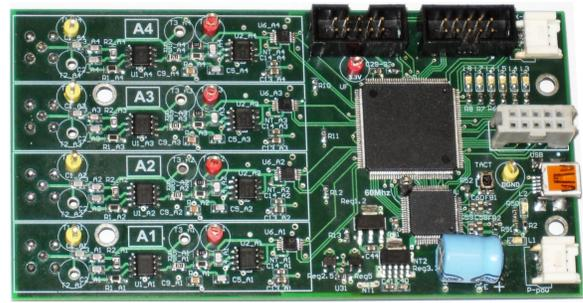
Figure 12: Hydrophone Amplification/Processing Hardware
