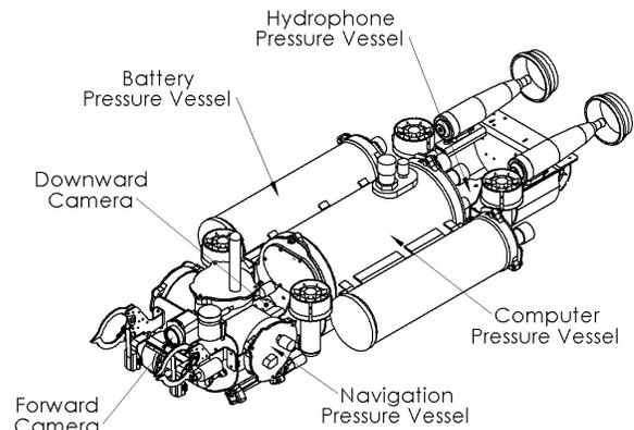
Figure 1: Assembly of SubjuGator 7 Pressure Vessels
