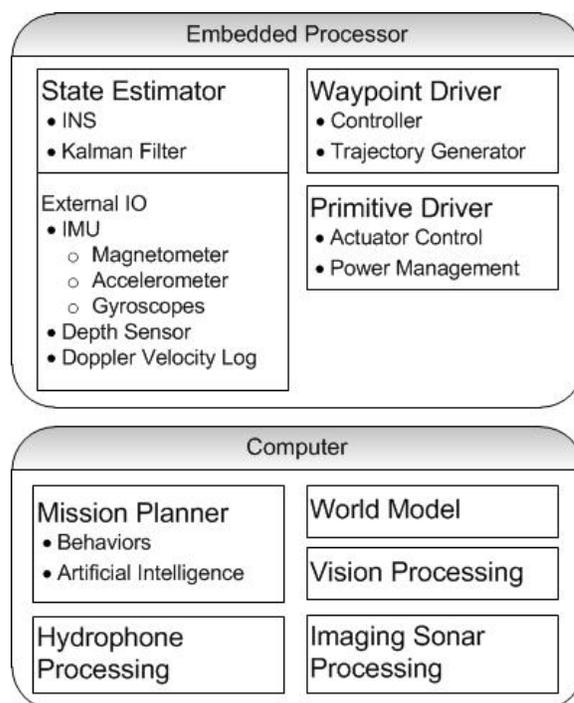
Figure 15: Software High Level Block Diagram
