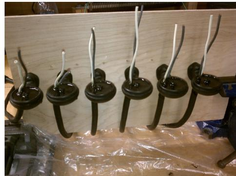
Figure 4: Custom cable potting for thrusters
