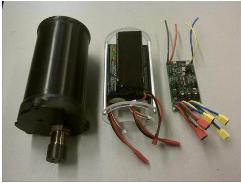
Figure 10: Battery pod pressure vessel and internal configuration.
