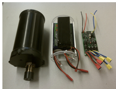
Figure 10: Battery pod pressure vessel and internal configuration.
