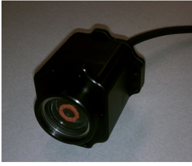
Figure 11: Camera pressure vessel assembled with Point Grey camera.
