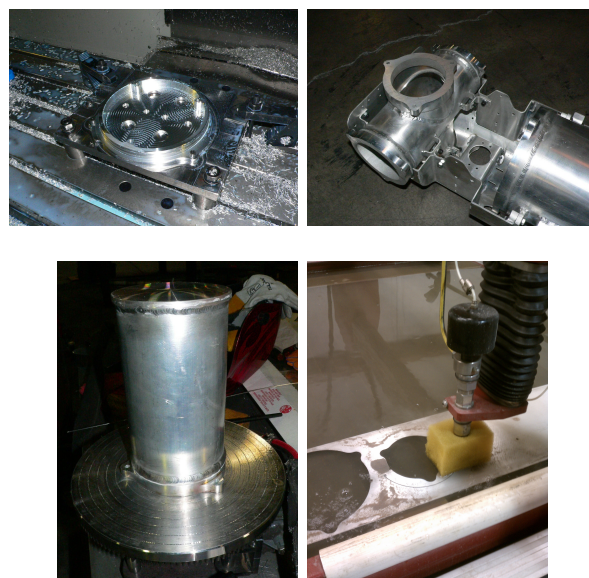
Figure 3: Top Left: CNC machining of an endcap, Top Right: DVL box in the main frame, Bottom Left: Welding of a battery pod, Bottom Right: Waterjet cutting.
