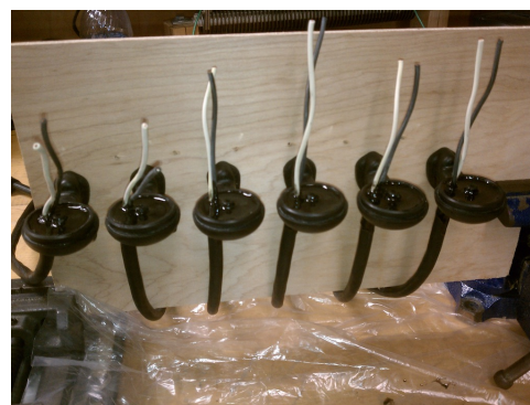
Figure 4: Custom cable potting for thrusters.
