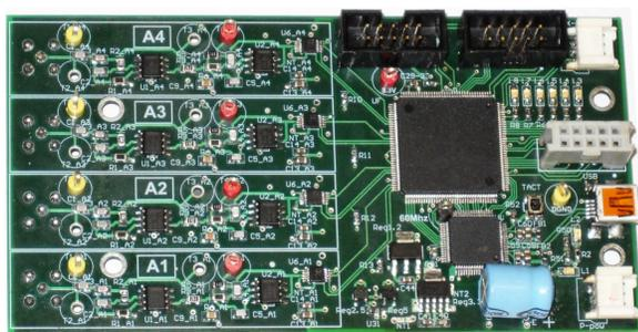
Figure 12: Passive sonar amplification and processing hardware.
