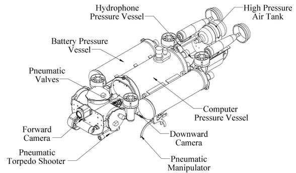
Figure 1: Assembly of SubjuGator 7 pressure vessels.
