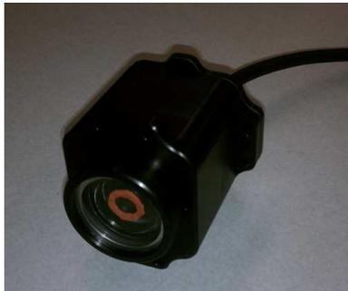
Figure 11: Camera pressure vessel assembled with Point Grey camera.
