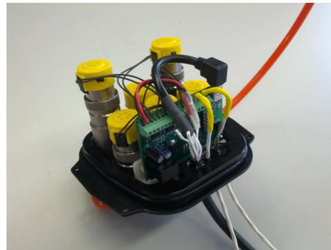
Figure 13: Pneumatic solenoid valve housing and control board.
