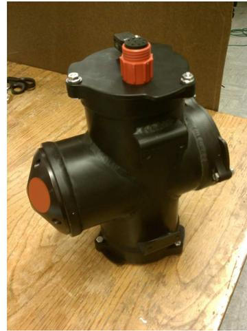
Figure 9: Navigation pressure vessel.
