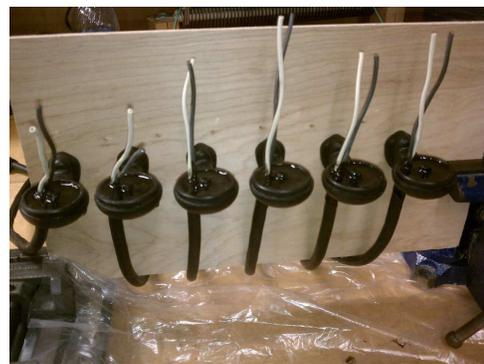
Figure 4: Custom cable potting for thrusters.
