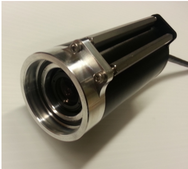
Figure 11: Camera pressure vessel assembled with uEye camera.
