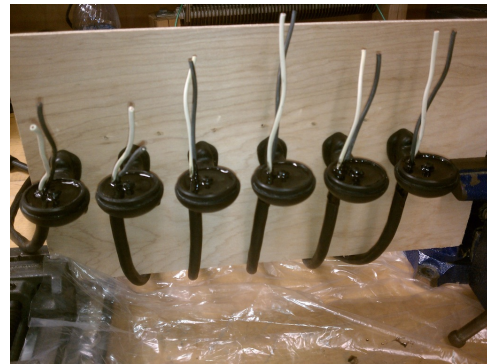
Figure 4: Custom cable potting for thrusters.
