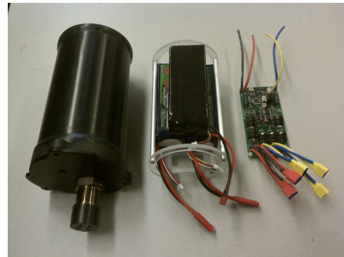
Figure 10: Battery pod pressure vessel and internal configuration.
