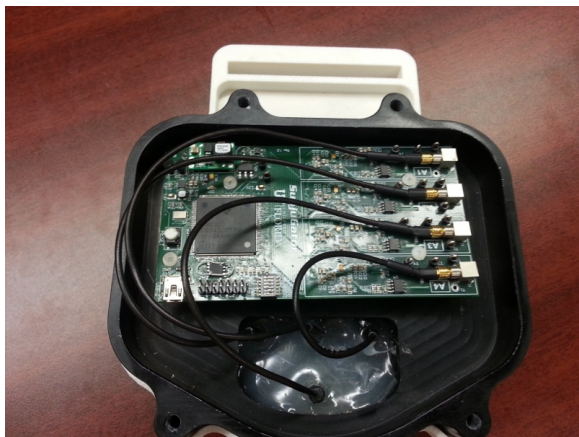
Figure 12: Passive sonar amplification and processing hardware.
