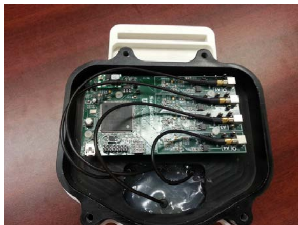
Figure 12: Passive sonar amplification and processing hardware.
