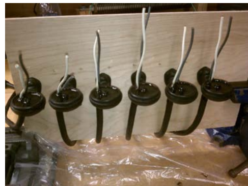
Figure 4: Custom cable potting for thrusters.
