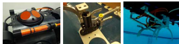
Figure 14: Left: Torpedo shooter, Middle: Ball dropper, Right: Manipulator assembly.
