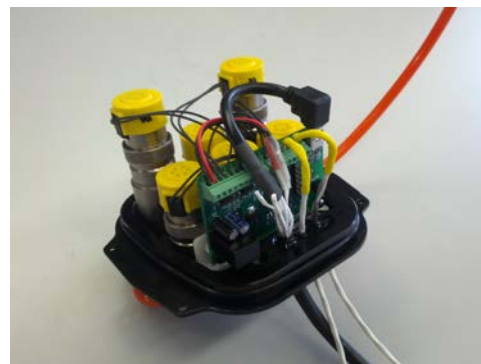
Figure 13: Pneumatic solenoid valve housing and control board.
