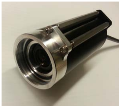
Figure 11: Camera pressure vessel assembled with uEye camera.
