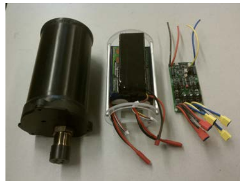
Figure 10: Battery pod pressure vessel and internal configuration.
