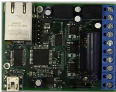
Figure 6: Motor control hardware.
