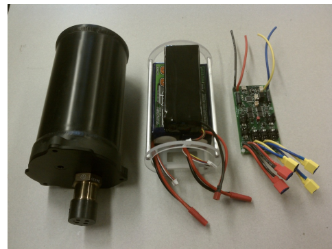
Figure 10: Battery pod pressure vessel and internal configuration.
