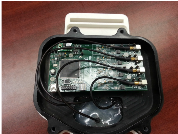
Figure 12: Passive sonar amplification and processing hardware.
