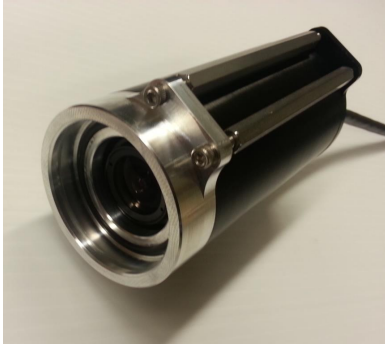
Figure 11: Camera pressure vessel assembled with uEye camera.
