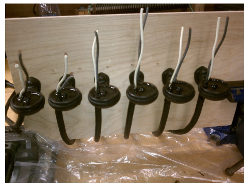
Figure 4: Custom cable potting for thrusters.
