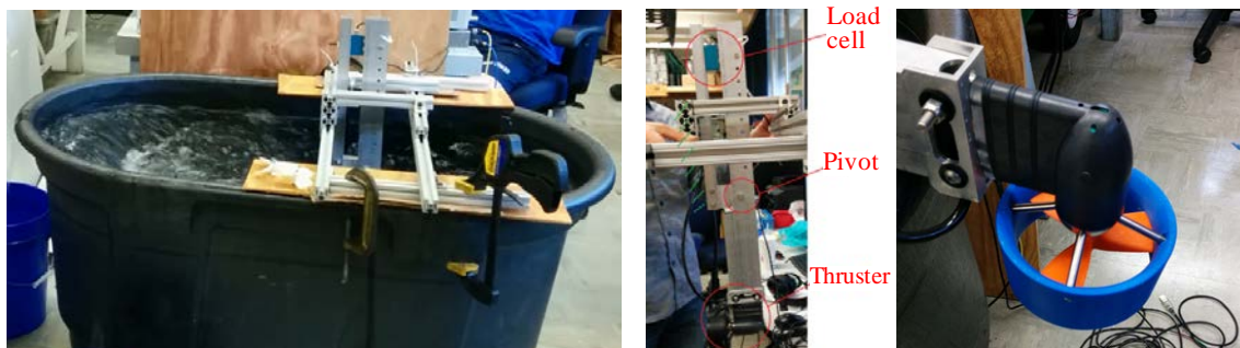
Figure 10: Thrust test (left), apparatus (middle), and current propeller and nozzle design (right).
