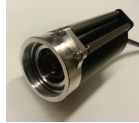
Figure 8: External camera pressure vessel with front endcap prior to anodization.
