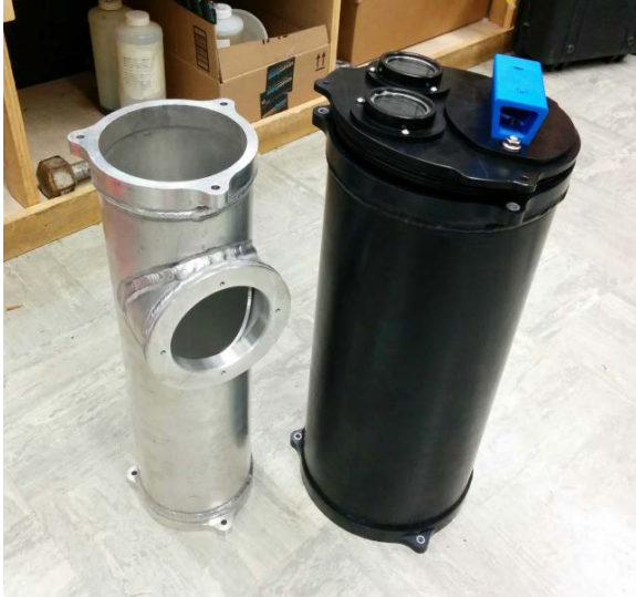
Figure 2: Navigation vessel before anodization (left) and main vessel with front endcap (right).
