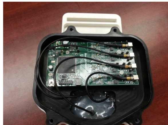
Figure 9: Passive sonar amplification and processing hardware.
