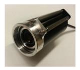
**Figure 8**: External camera pressure vessel with front endcap prior to anodization
