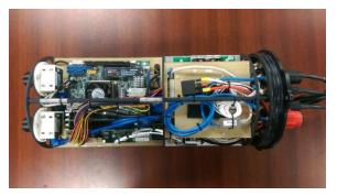
**Figure 4**: Internal electronics carriage for the main vessel. Above the tray there is easy access to PCBs and wiring, while batteries are stored below the tray
