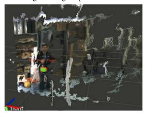
Figure 14: Stereo point cloud generation
