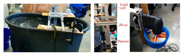
Figure 10: Thrust test (left), apparatus (middle), and current propeller/nozzle design (right)
