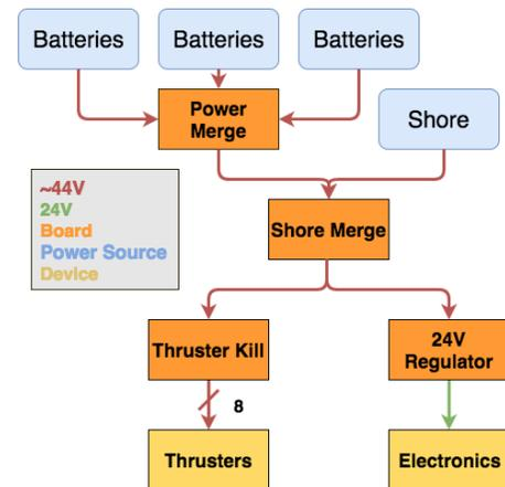
Fig 6. Power flow diagram.
