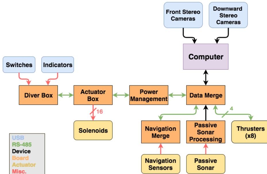
Fig 5. Communication flow diagram.
