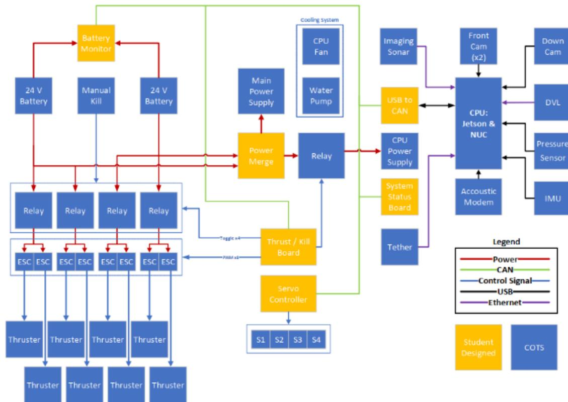
**Figure 5:** Electrical architecture.
